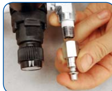
Connecting Gun to Air Compressor
