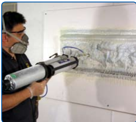
Spray urethane plastic to make fast, strong mother molds or castings.
