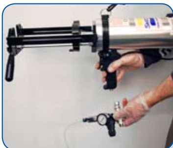
Attaching Air Pressure Regulator
