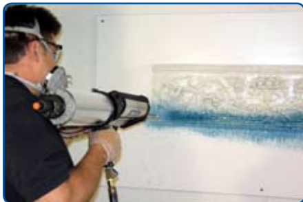
Spray urethane or silicone rubber for making molds of any original model.
