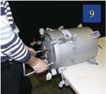
9 Position the lid on the pressure chamber.
