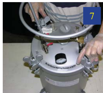
Be sure to secure the lid properly by tightening the wing nuts in tandem diagonally for best results.
