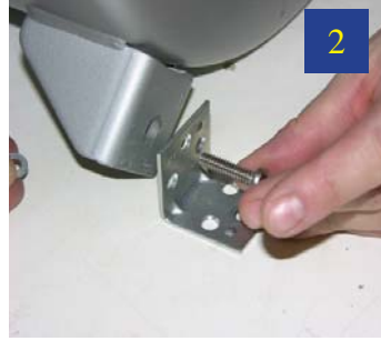
2 Use the enclosed hardware to attach the two brackets to the chamber.
