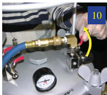
Flip the air control valve lever from the down position to the up position to release the air flow into the pressure chamber. Air will flow at 60 psi.
