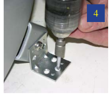
4 Use the self-starting screws to secure the chamber to the table top.
