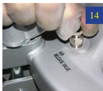
Keep the material under pressure for a duration at least equal to its demold time. Then release the air pressure valve.
