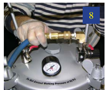
Attach an air supply hose. The regulator is preset at recommended 60 psi.
