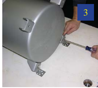
3 The chamber should be positioned so it extends slightly out over the table edge.
