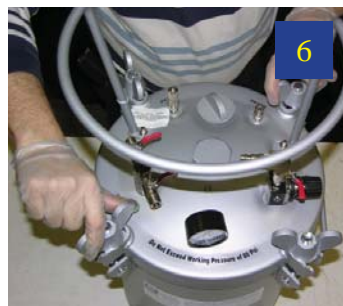
Be sure to secure the lid properly by tightening the wing nuts in tandem diagonally for best results.
