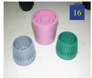
The result is a bubble-free casting that is identical to the original model.
