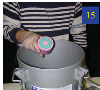
When the demold time is up, remove the mold from the pressure chamber.
