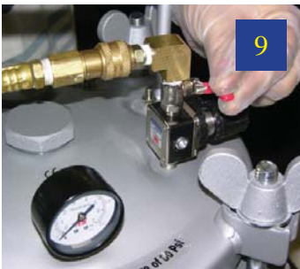
Flip the air control valve lever from the down position to the up position to release the air flow into the pressure chamber. Air will flow at 60 psi.
