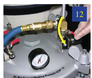
Close the air control valve by placing the valve in the down position.
