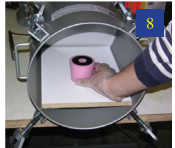
8 Place the resin-filled mold inside the pressure pot on the level board.
