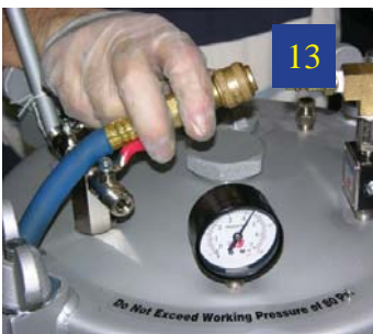
The air hose can then be removed and the chamber will retain its pressure.
