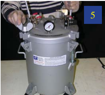
Place the lid on the pressure chamber and tighten the wing nuts.
