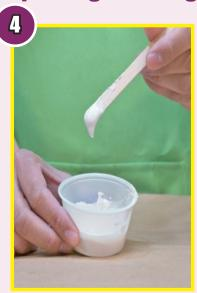
Dispense a small amount of LiquiStone<sup>TM</sup> and mix a tiny amount of water into it to create a paste.
