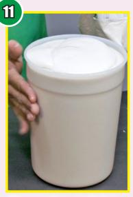
After pouring, gently tap the side of the bucket to help settle the LiquiStone™ in the mold. Allow LiquiStone™ to set for 3 hours at room temperature (73°F/23°C).
