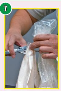
After mixing, grab one corner of the bag and cut it off so the mixed material can be poured easily into the mold.
