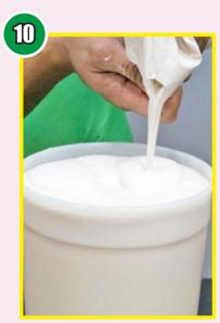
Set the mold down and continue pouring the LiquiStone™ to fill to the top of the bucket.
