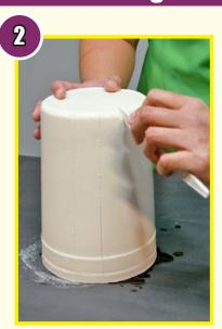
To facilitate demolding, use a plastic knife to carefully score the alginate mold on all sides. Carefully remove small chunks of alginate to reveal the casting.
