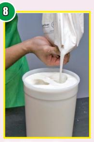
Carefully pour the LiquiStone™ into the mold. Fill the mold cavity about half way and stop.
