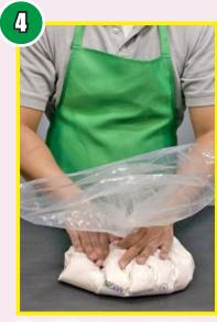
Unroll the bag and grip tightly at the top of the LiquiStone™. Roll in a circular motion to circulate water through the LiquiStone™.
