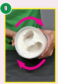
Pick up the mold and rotate in all directions for about 10 seconds to help minimize air entrapment in the finished casting.
