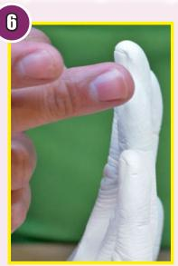
Use your finger to smooth and wipe away any excess material. Repaired area cures in 3 hours.
