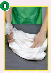
Use the flat side of your palm to aggressively mix the LiquiStone™ by pressing and kneading the bag against the surface of the table.
