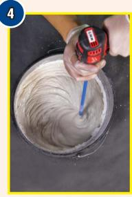
Mix the alginate and water using a turbine mixer and a variable speed drill.
