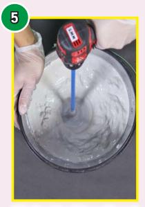
Mix the LiquiStone<sup>™</sup> and water using a turbine mixer and a variable speed drill.
