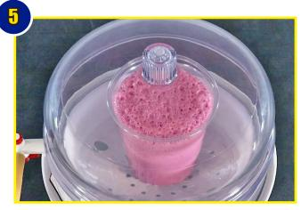
Observe material as it expands under vacuum. The material will rise, so be sure the container is large enough to accomodate the expansion! If material looks like it's going to overflow, release pressure using the valve.
