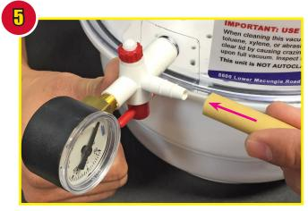
Attach the Rubber Vacuum Hose to the Valve Assembly as shown to secure in position.
