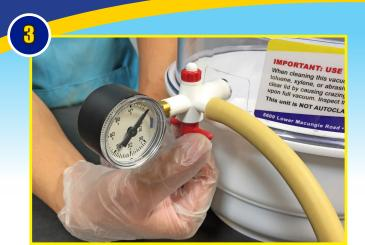
Turn the Valve a quarter turn to open and draw vacuum into the Vacuum Chamber.
