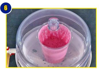
After material collapses, wait about 60 seconds before turning off the Vacuum Pump. Turn the Valve to release the vacuum from the chamber. Once the vacuum has been released from the chamber, open the lid and remove the degassed material.
