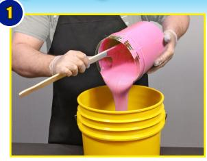
Dispense and mix material according to instructions. Pour material into a new container that is large enough to contain the rise of material during vacuuming (up to 5x expansion).
