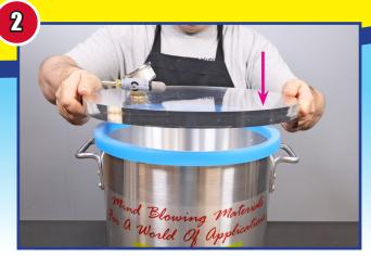
Place the Clear Vacuum Chamber Lid onto the Chamber.
