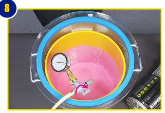
After material collapses, wait about 60 seconds before turning off the Vacuum Pump. Turn the Valve to release the vacuum from the chamber. Once the vacuum has been released from the chamber, open the lid and remove the degassed material.
