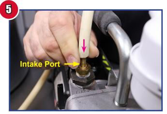
Attach the other end of the Rubber Vacuum Hose to the Intake Port on the Vacuum Pump. Push the Rubber Vacuum Hose down to secure in position.
