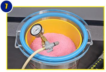
**IMPORTANT:** Do not walk away! Always monitor the rise of material. Use the valve to prevent it from going too high and into the air intake port.
