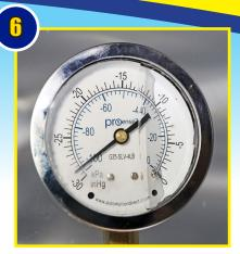
Vacuum should pull 29" of Mercury (1 Bar) in the chamber for proper degassing.
