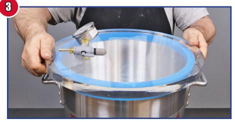
Check that the Clear Chamber Lid is centered on the chamber in order to create a tight seal.
