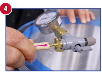
Attach the Rubber Vacuum Hose to the Valve Assembly as shown to secure in position.
