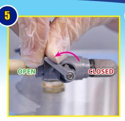
Turn directional Valve to open position and draw vacuum into the Vacuum Chamber.
