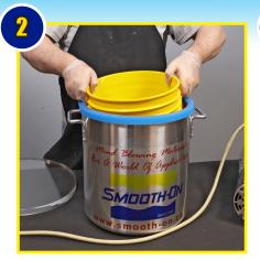
Place container with material into the Vacuum Chamber.
