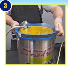
Center the Chamber Lid on top of the Blue Gasket to create an air tight seal.
