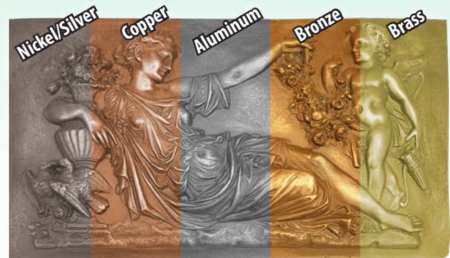
Smooth-Cast™ ONYX™ is combined with different metal powders to achieve a realistic metal finish.
