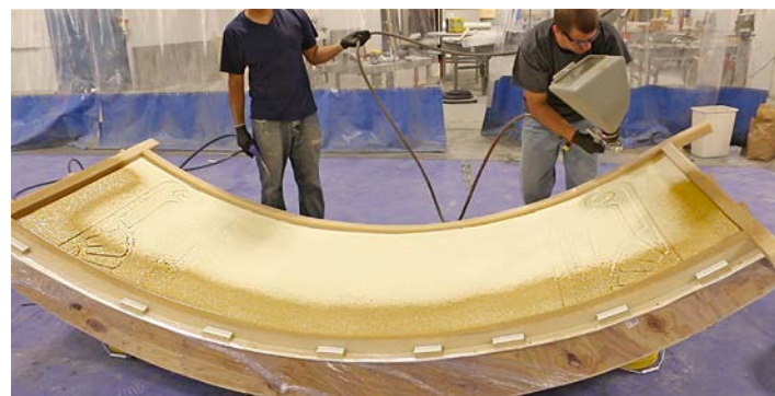
5 The GFRC face mix is sprayed using a hopper gun.
