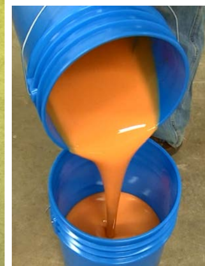
3 PMC®-780 is pigmented and drill mixed.
