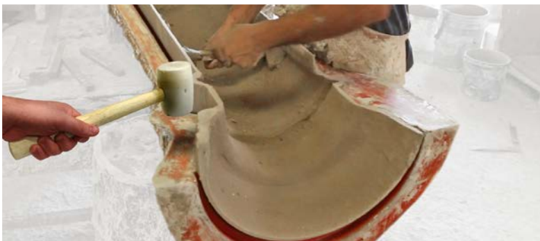
5 Forton® MG elements can be demolded after 60-90 minutes.
