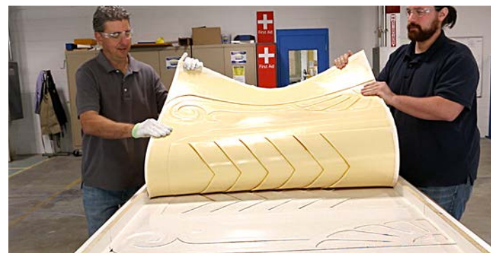
4 After curing for 16 hours, the rubber liner is demolded.
