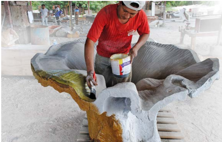
8 A multi-step staining process makes the GFRC casting look exactly like the original.
