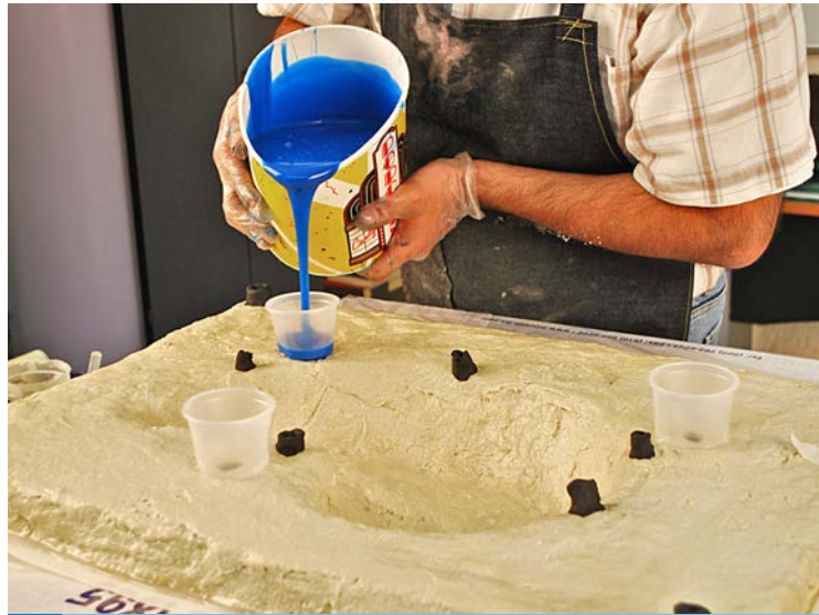
4 Mold Star® 30 silicone is mixed and poured into the cavity mold.
