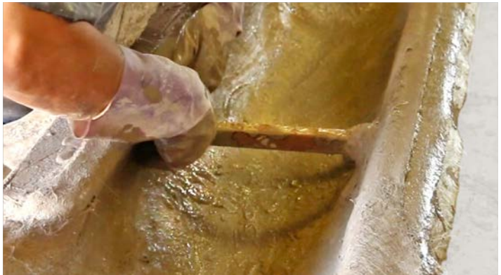
4 Wood supports are embedded in the back of the casting for attachment points.
