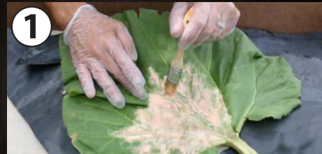
Multiple Layers of Rebound® 25 mold rubber are applied to a leaf.
