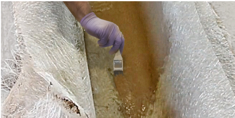
3 Alternating layers of Forton® MG and E-glass veil are applied to build up to the desired thickness, typically 3/8" (10 mm).
