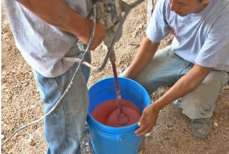
2 Rebound® 25 mold rubber is dispensed 1A : 1B by volume. A drill mixer is used to thoroughly mix the two parts.
