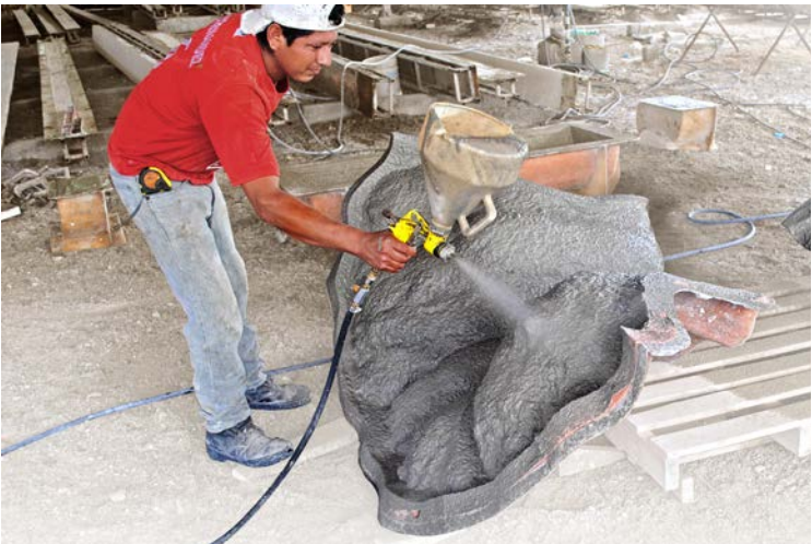
5 GFRC is sprayed into the mold halves. Mold halves are then put together.
