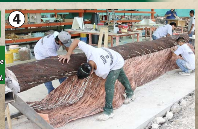
The rubber is allowed to cure for 6 hours before demold.
