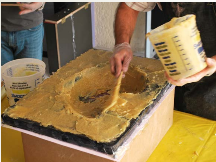
3 Plasti-Paste® II urethane plastic is applied to form the first half of the rigid support shell.
