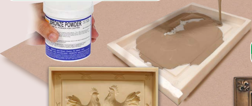
1 A gel coat mixture of FORTON® MG and bronze powder is applied to the mold surface.
