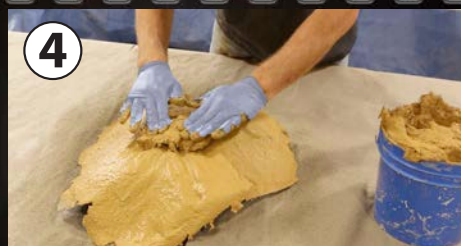
Layers of GFRC are applied to the mold.
