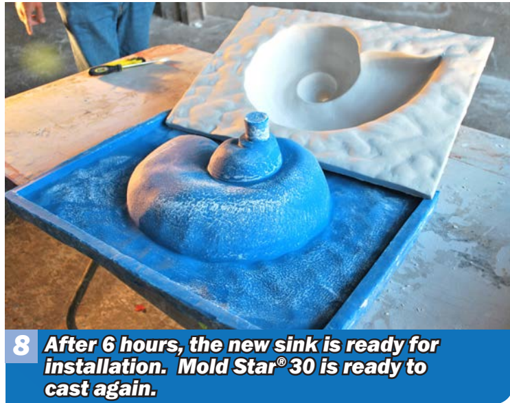
6 Mold Star® 30 captures perfect detail and the mold is ready for polymeric concrete casting.
