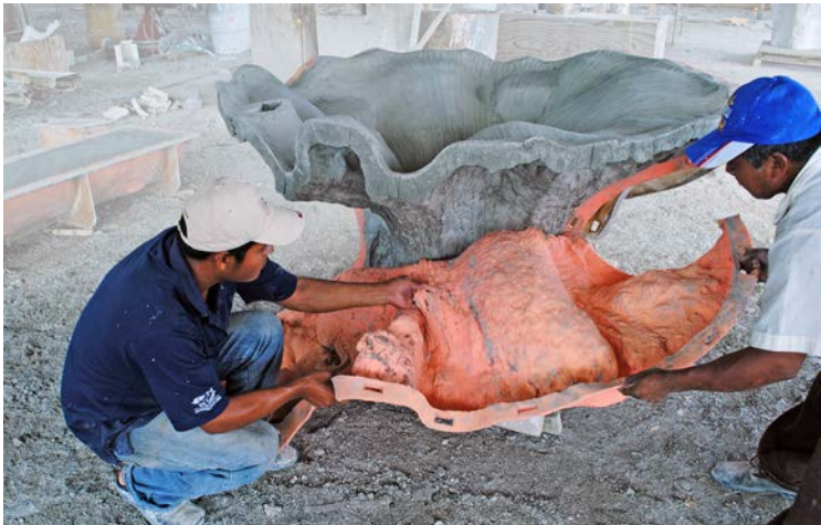
7 Finished GFRC casting is removed from the Rebound® 25 rubber mold.
