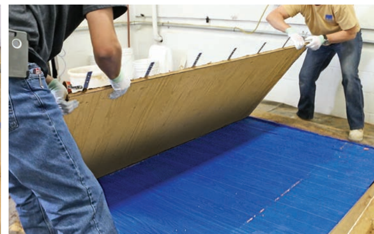
8 Four GFRC panels of different sizes will be made from the same mold
