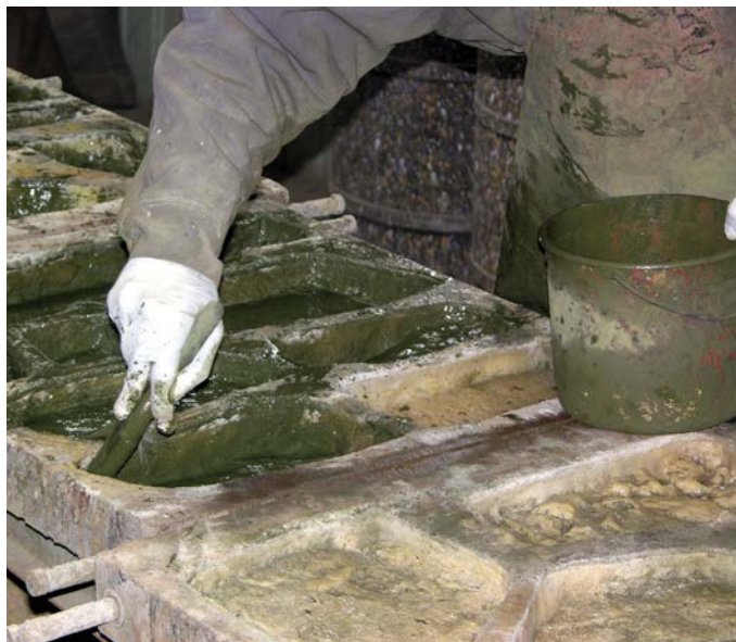
2 Mold cavity is pigmented to desired color.
