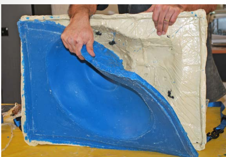
5 Mold Star® 30 cures in 6 hours and the other half of the cavity mold is poured.
