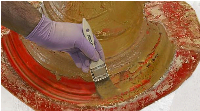
1 A facecoat of Forton® MG is brushed onto the mold surface.
