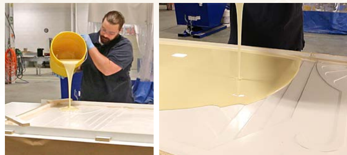
3 VytaFlex® 60 is properly measured, mixed and poured over the entire model.
