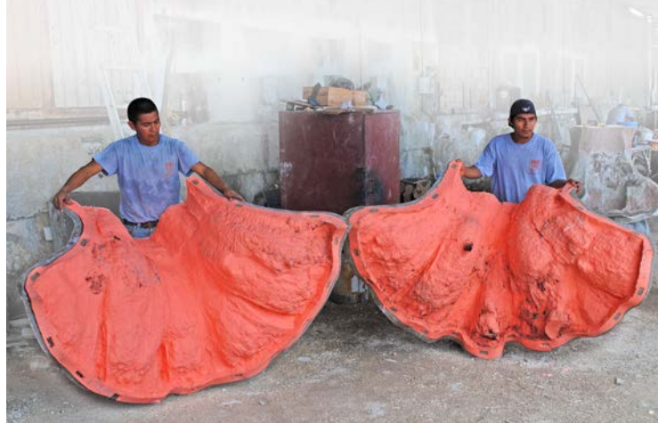
4 A support shell is applied, allowed to cure and then removed. The rubber mold is removed from the original and ready for GFRC casting.
