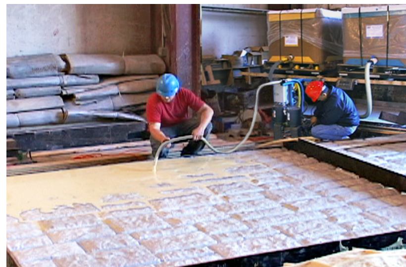
1 VytaFlex® 60 mold rubber is meter mix dispensed.
