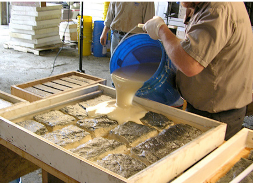
1 VytaFlex® 60 mold rubber is mixed and poured into the mold box.
