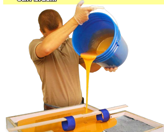
4 Rubber is poured onto the pavers, ensuring straps are embedded within the PMC®-780.
