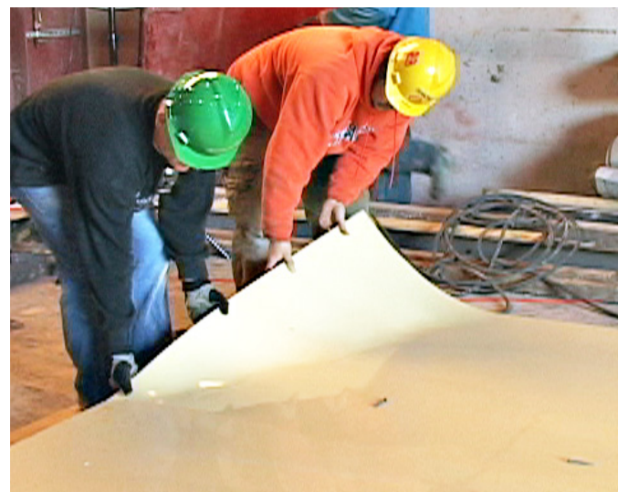
2 Rubber is allowed to cure and is demolded.
