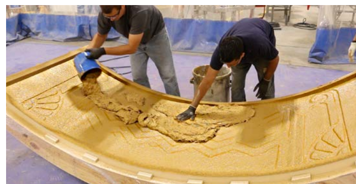
6 The GFRC backer mix (with AR glass fiber) is then applied.
