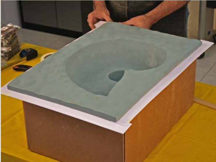
1 A CNC model is sealed with grey primer in preparation for mold making.
