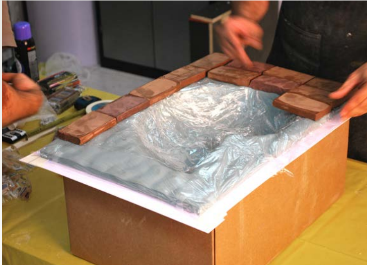
2 A cavity pour mold making technique is used to create the mold. Sulfur-free modeling clay is used to form the cavity.
