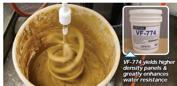
5 GFRC components are mixed in a high-shear mixer.
