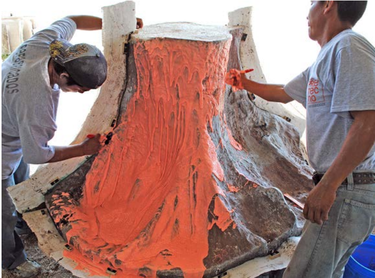
3 The mold is made in 2 halves, each consisting of 4 brush-on layers.
