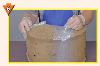
Cut a pour hole over the area to be repaired with an exacto knife.
