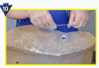
Apply packing tape over the pour hole to seal it. Tape will release as the foam expands through the pour hole.
