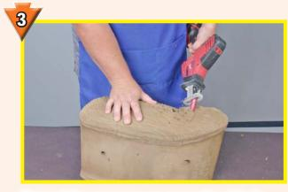
Repeat the process on opposite side to remove damaged and loose foam.
