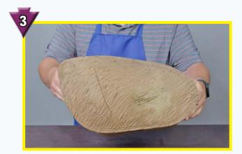
Repair to the front side of the core is complete. FlexFoam-iT!<sup>™</sup> 15 permanently bonds to the original foam.
