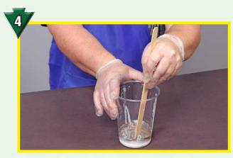
Transfer both Part B containers into a larger mixing container. Add UVO<sup>™</sup> colorants to Part B as before and mix thoroughly.
