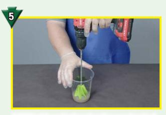
Add Part A and mix using the mechanical mixer and drill. **FlexFoam-iT!™ 15 has a 2 minute potlife**, so work quickly to thoroughly mix the material.
