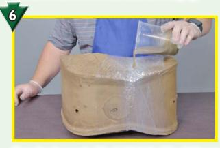
Repaired area is filled 1/3 full of liquid foam. Foam will expand 4 times its original volume. After pouring the foam, apply packing tape over the pour hole to seal it.
