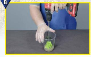
Mix with the mechanical mixer and drill. Start at a slow speed and increase to a high speed to mix the foam. FlexFoam-iT!™ 15 has a 2 minute potlife, so work quickly to thoroughly mix the material.
