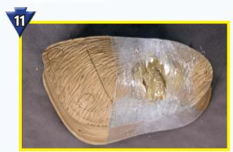
Allow FlexFoam-iT!<sup>™</sup> 15 to cure for 4 hours at room temperature (73°F/23°C).
