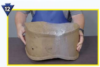
After foam cures, flip the core over to prepare the second side for repair.
