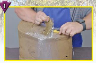
After foam is allowed to cure for 4 hours, trim excess foam off with a breakaway razor utility knife.
