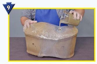
Repaired area is filled 1/3 full of liquid foam. Foam will expand 4 times its original volume.
