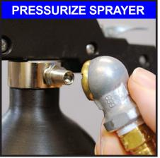
Charge sprayer with compressed air using a standard air chuck. Hold air chuck on valve stem until you hear the line pressure equalize with the sprayer.
