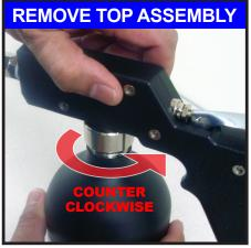
2. Once sprayer has been depressurized remove the top unit by turning it counterclockwise while holding the canister firmly.
