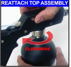
Screw top assembly onto canister in a clockwise direction. Make sure assembly has been fully seated.
