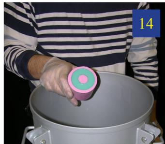
14 When the demold time is up, remove the mold from the pressure chamber.
