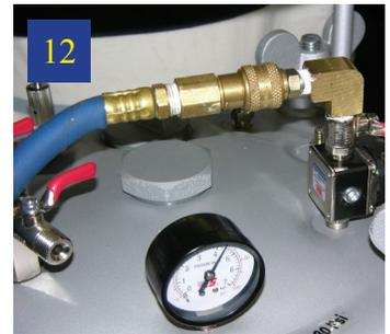
12 Keep the air supply connected and the material under pressure for a duration at least equal to its demold time.
