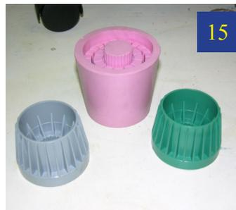
15 The result is a bubble-free casting that is identical to the original model.
