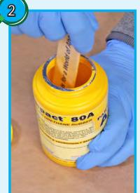
Pre-mix Part A – Open container and thoroughly pre-mix the material using a clean mixing stick. Be sure to scrape the sides and bottom as you mix.
