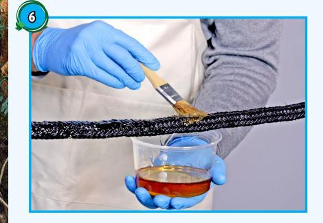
Brush Simpact<sup>™</sup> 80A-II mixture onto the marine rope using a clean, disposable brush, completely covering top and sides of the rope.
