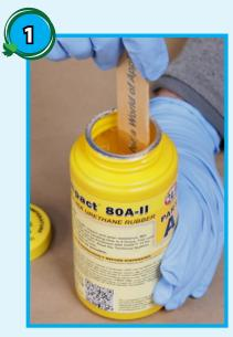
**Pre-mix Part A** – Open container and thoroughly pre-mix the material using a clean mixing stick. Be sure to scrape the sides and bottom as you mix.
