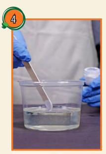
Add **UVO™** colorants to Part A to reach desired base color in the mixture. In this example, begin by adding a base white to the mixture. Mix the pigment thoroughly.
