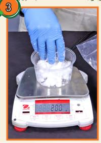
Measure 10% URE-FIL<sup>™</sup> 13 by weight of the measured Part A of the Simpact<sup>™</sup> 80A mixture. In this example, measure out 20gURE-FIL<sup>™</sup> 13.
