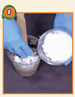
Add URE-FIL<sup>™</sup> 13 to the mixture and mix thoroughly. Be sure to scrape the sides and bottom of the container as you mix the material.
