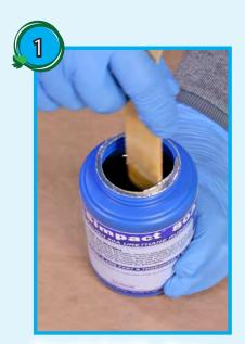
Pre-mix Part B – Open container and thoroughly pre-mix the material using a clean mixing stick. Be sure to scrape the sides and bottom as you mix.
