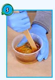
Dispense Parts A and B into a clean mixing container and mix thoroughly. Scrape the sides and bottom of the mixing container several times. Pour the mixture into another clean container and mix again.
