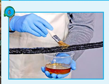
Brush Simpact™ 80A mixture onto the marine rope using a clean, disposable brush, completely covering top and sides of the rope.
