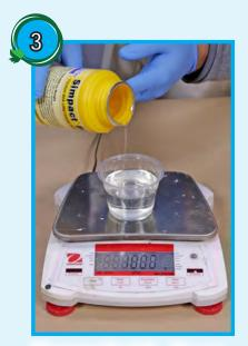
Measure Part A – Use an accurate gram scale to measure out 100g of Part A by weight. The mix ratio of Simpact™ 80A is 100A to 60B.
