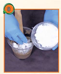
Add URE-FIL<sup>™</sup> 13 to the mixture and mix thoroughly. Be sure to scrape the sides and bottom of the container as you mix the material..
