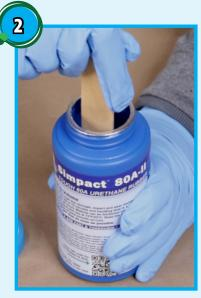
**Pre-mix Part B** – Open container and thoroughly pre-mix the material using a clean mixing stick. Be sure to scrape the sides and bottom as you mix. It is important to thoroughly pre-mix Part A and Part B BEFORE dispensing the material!
