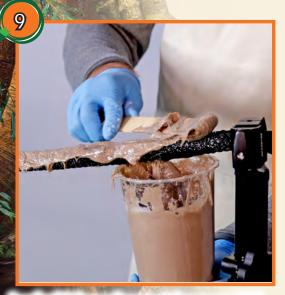
Apply thickened material approx .25" (6.4mm) to .5" (12.7mm) thick onto rope with a paint stick. Cover all sides. Rotate rope 180 degrees so that the bottom surface of rope is now on top, and then add thickened resin to this area.
