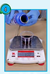
Measure Part B – Use an accurate gram scale to measure out 60g of Part B by weight. The mix ratio of Simpact™ 80A is 100A to 60B.
