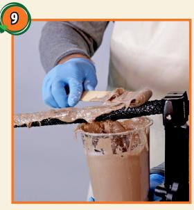
Apply thickened material approx 0.25" (6.4mm) to 0.5" (12.7mm) thick onto rope with a paint stick. Cover all sides. Rotate rope 180 degrees so that the bottom surface of rope is now on top, and then add thickened resin to this area.
