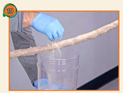
After coating all sides of the rope with thickened material, sprinkle play sand onto the surface. Adding play sand will prevent the material from sticking to texture stamps, sculpting tools, and provide a matte surface finish. Let the material cure for 10-15 min. Additional layers maybe added if desired.
