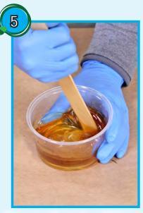
Dispense Parts A and B into a clean mixing container and mix thoroughly. Scrape the sides and bottom of the mixing container several times. Pour the mixture into another clean container and mix again.
