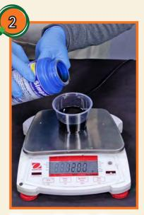
Measure Part B – Use an accurate gram scale to measure out 120g of Part B by weight. The mix ratio of Simpact™ 80A is 100A to 60B.
