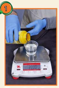
Measure Part A – Use an accurate gram scale to measure out 200g of Part A by weight. The mix ratio of Simpact™ 80A is 100A to 60B.
