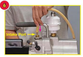
Attach the other end of the Rubber Vacuum Hose to the Intake Port on the Air Compressor. Push the Rubber Vacuum Hose down to secure in position.
