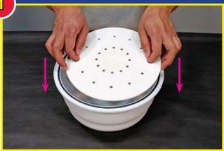
Insert Chamber Overflow Plate into the Vacuum Chamber Bowl. Make sure the plate is level.
