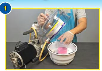
Place material to be vacuum degassed into the Vacuum Chamber Bowl and close the Chamber Lid to create an air tight seal.
