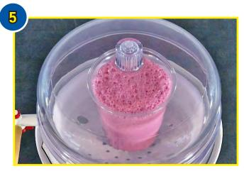
Observe material as it expands under vacuum. The material will rise, so be sure the container is large enough to accomodate the expansion!
