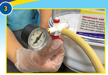
Turn the Valve a quarter turn to open and draw vacuum into the Vacuum Chamber.
