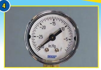
Vacuum should pull 29" of Mercury (1 Bar) in the chamber for proper degassing.
