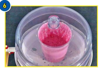
After material collapses, wait about 90 seconds before turning off the Air Compressor. Turn the Valve to release the vacuum from the chamber. Once the vacuum has been removed from the chamber, open the lid and remove the degassed material.
