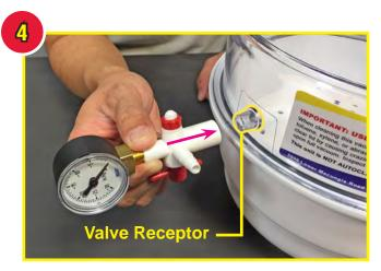
Use gentle pressure to attach the Valve Assembly to the Chamber Lid Valve Receptor located on the side of the Chamber Lid. (highlighted in photo above.)
